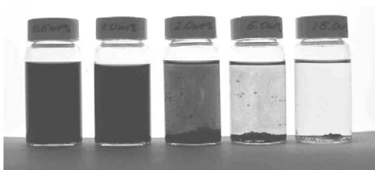
Fig. 11. Dissolving experiments on nanotube filled polycarbonates after 2 weeks in THF, from left to right: 0.5, 1, 2, 5, and 15 wt% composites.
